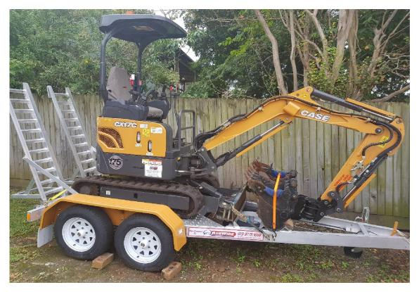
Featuring a Calibre Power-tilt quick hitch, changing and tilting each attachment through 180 degrees of range is quick and easy, requiring no safety pin.
