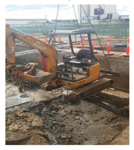
Featuring adjustable tracks and a quickly removable ROPS canopy, this machine can readily be used in tight spaces down to 1.5 metres in height and under 1 metre in width.
