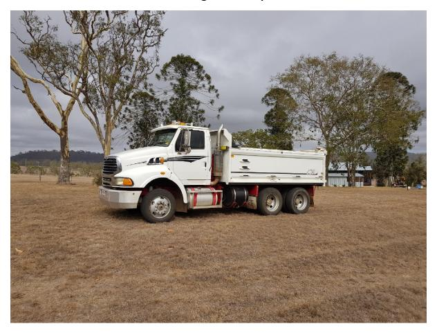
With a heavy-duty Hardox body and light tare-weight, our Sterling tipper is able to legally carry payloads of 12.5 Tonnes. Because of the heavy-duty body we are able to carry all types of loads including shot-rock and demolition waste. For use on jobsites with higher safety standards, we have fitted large Fire extinguishers in and out of the cab, an 80-channel two-way radio, flashing beacon, first aid kit and more...
