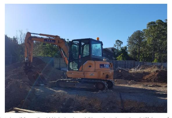
Featuring a JB Power-tilt quick hitch, changing and tilting each attachment through 180 degrees of range is quick and easy, requiring no safety pin.
